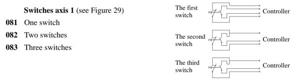
Figure 29 Connections of the switches
