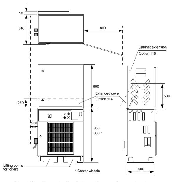
Figure 10 View of the controller from the front and from above (dimensions in mm).
