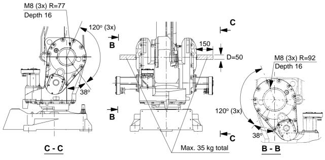
Figure 20 The shaded area indicates the permitted positions (centre of gravity) for any extra equipment mounted in the holes (dimensions in mm).
