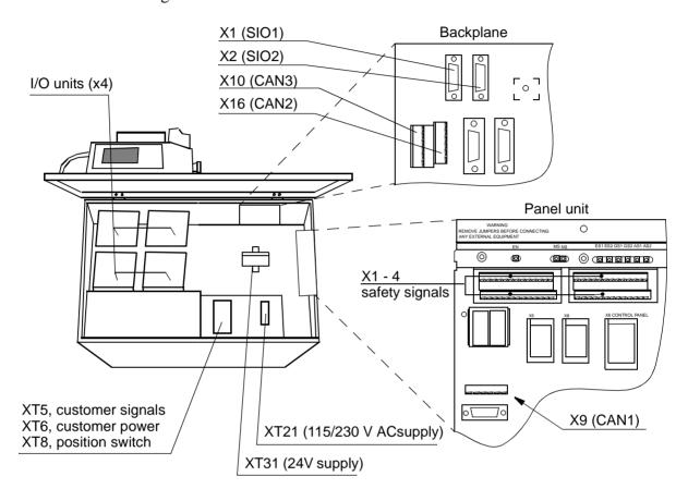
Figure 38 I/O unit and screw terminal locations.
