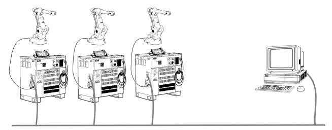
Figure 27 Serial network communication.
