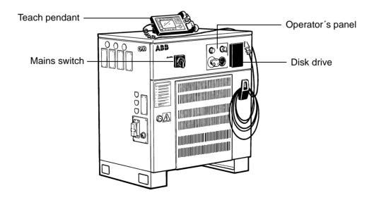
Figure 2 The controller is specifically designed to control robots, which means that optimal performance and functionality is achieved.
