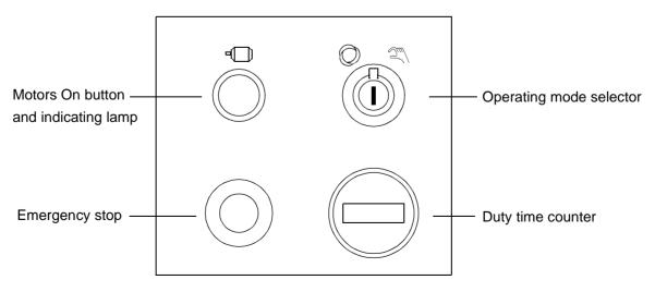
Figure 5 The operating mode is selected using the operator's panel on the controller.
