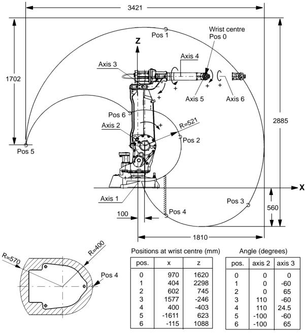
Figure 23 The extreme positions of the robot arm (dimensions in mm).
