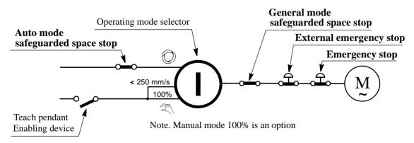
Figure 13 All safeguarded space stops force the robot's motors to the MOTORS OFF state.
