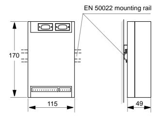
Figure 40 Dimension for units 67U-Z, 69A-B.
