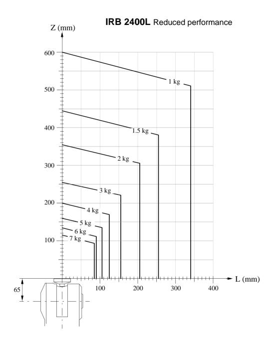
Z = see the above diagram and the coordinate system in Figure 9
