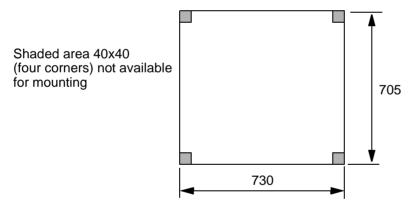
Figure 33 Mounting plate for mounting of equipment (dimensions in mm).
