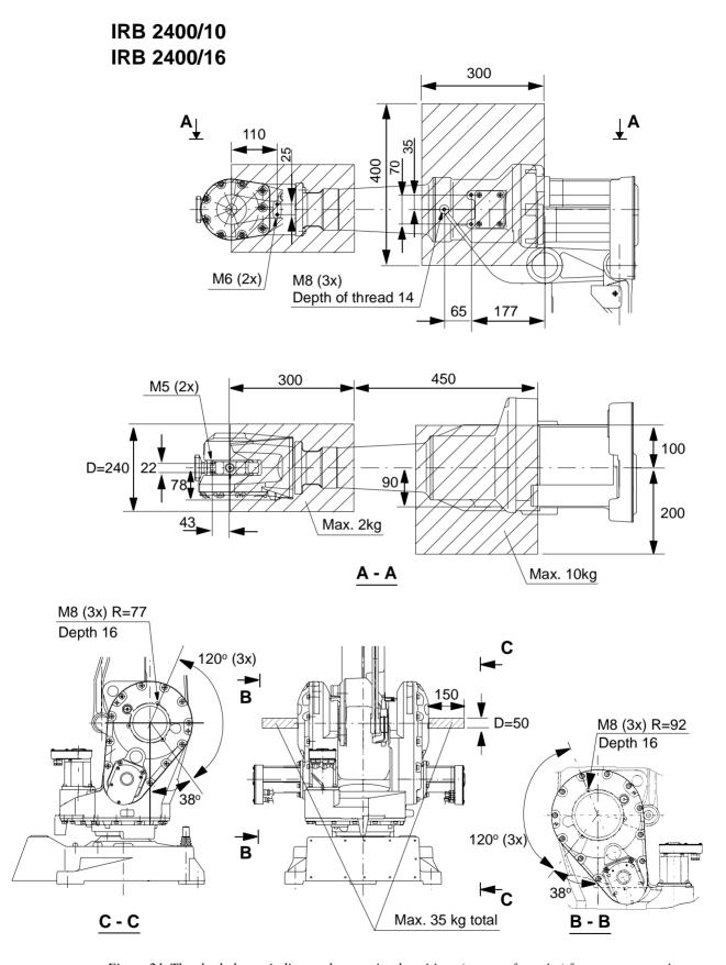
Figure 21 The shaded area indicates the permitted positions (centre of gravity) for any extra equipment mounted in the holes (dimensions in mm).
