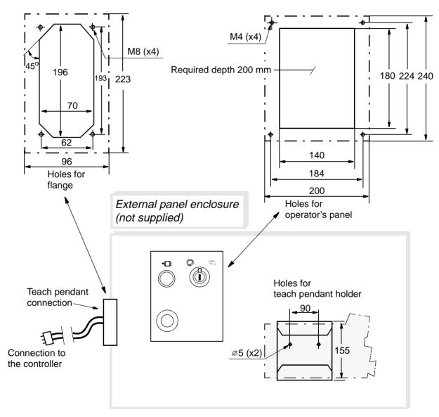
Figure 34 Required preparation of external panel enclosure (all dimensions in mm).
