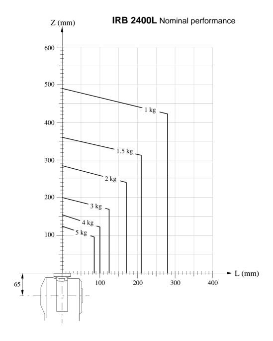
Z = see the above diagram and the coordinate system in Figure 9
