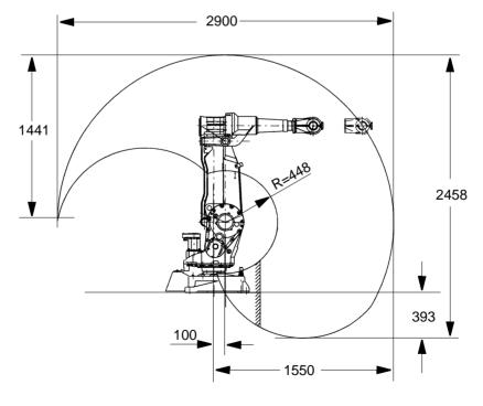
Figure 8 Working space of IRB 2400 (dimensions in mm).
