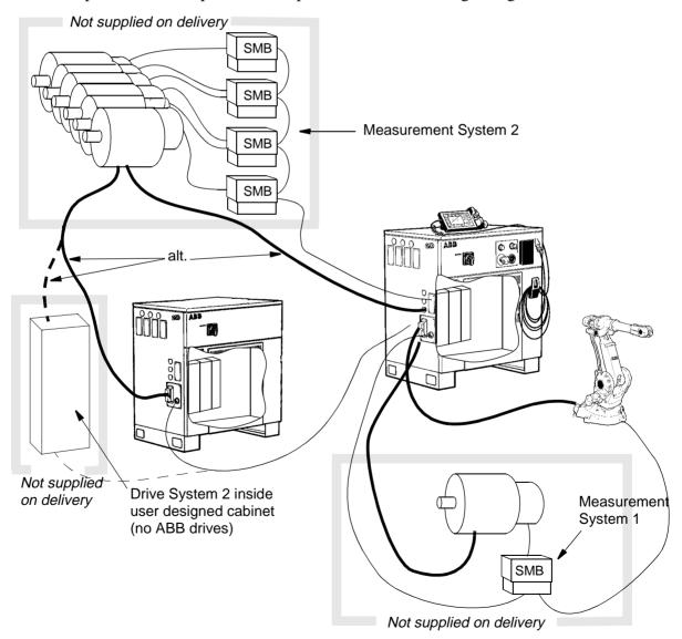
Figure 25 Outline diagram, external axes.
