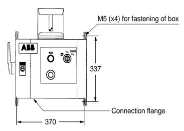
Figure 35 Operator's panel mounted in a box (all dimensions in mm).
