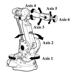
Figure 1 The IRB 2400 manipulator has 6 axes.
